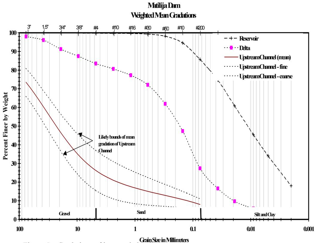
Figure 5 – Gradations of impounded sediments
