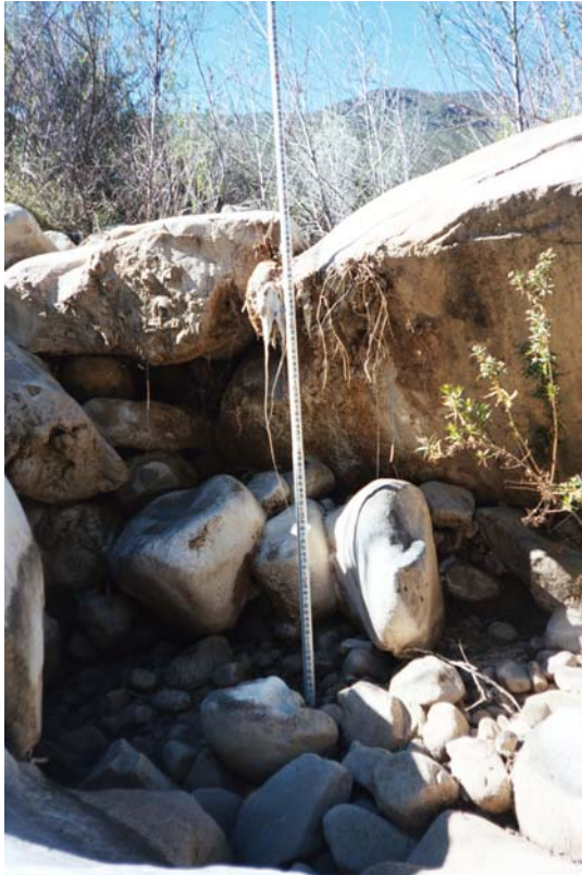
Barrier #65 in Old Man Creek. Visible portion of stadia rod is approximately 11 ft long. See Figure 3 for location and Table 2 for barrier details.
